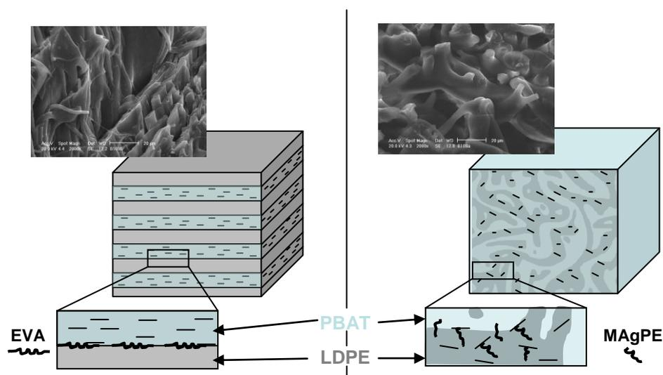
Depending of the compatibilizer, it has been found that the nanoclay can be selectively located in either the polyolefinic or polyester phase while the interphase is invariably stabilized by clay platelets. Remarkably enough, such a selection allows controlling the morphology of the polymer blends. The mechanical properties of the polymer blends were interpreted in the light of their morphology.
