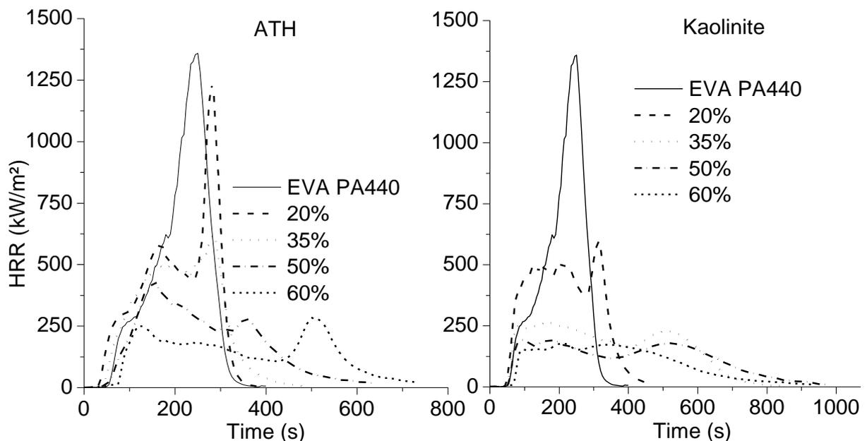
Fig. 1. Cone calorimeter results at  $50 \text{ kW} \cdot \text{m}^{-2}$ .
