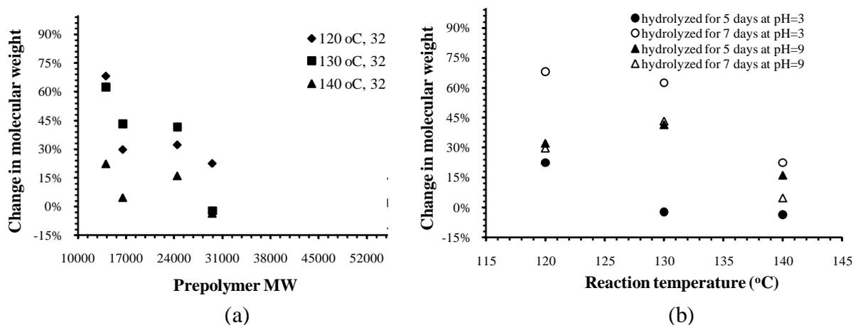
Fig. 1. a) Change in molecular weight after 32 h of SSP of both grades, b) change in molecular weight vs. reaction temperature for prepolymers of MW < 30,000 g mol<sup>-1</sup>.
