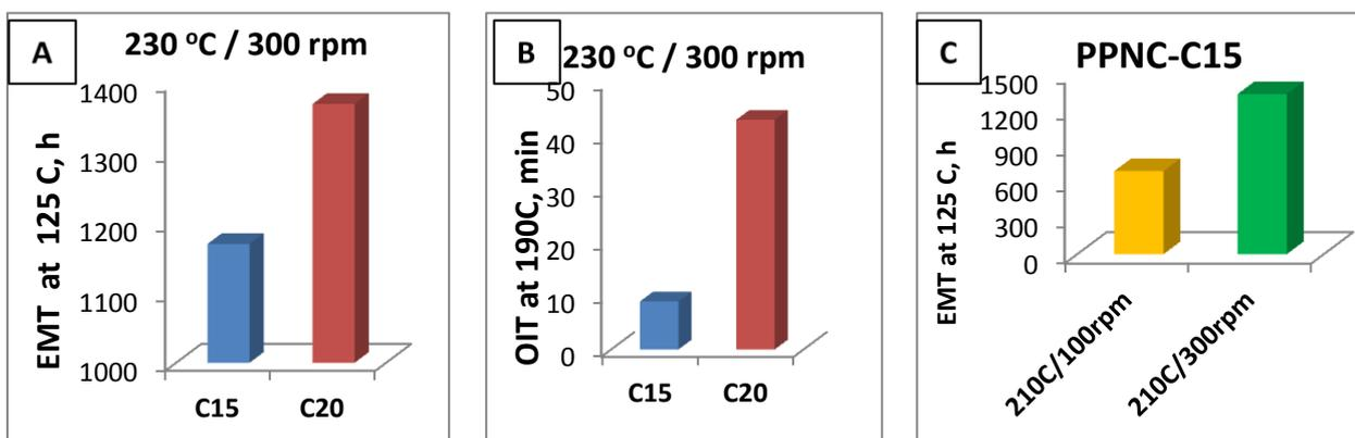
**Fig. 2.** Time-to-embrittlement from LTTs tests of PPNCs produced under different extrusion conditions.
