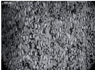
Fig. 1. Microstructure of LDPE foam
