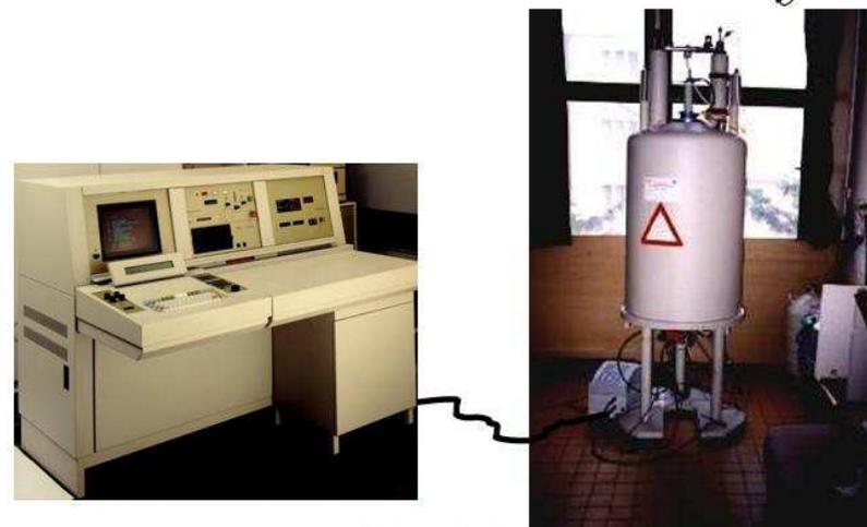
NMR spectrometer with a cryomagnet.
