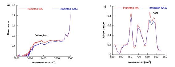
**Figure 2:** FTIR spectra of industrial PVC film irradiated at room temperature under air and followed at room temperature (in red) and at 120°C (in blue) under inert atmosphere: a) OH region b) C-Cl region.
