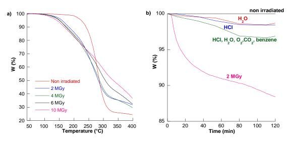
**Figure 1:** Thermal decomposition of PVC: a) Dose effect, b) Isothermal weight loss and HCl and water formation at 120°C.
