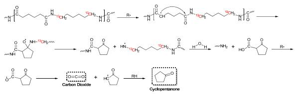
**Figure 2.** One possible thermal-oxidative degradation mechanism of nylon 6.6 within the nylon backbone that leads to the formation of cyclopentanone; alternatives may exist, e.g. the removal of the carboxylic group through a non-radical reaction.
