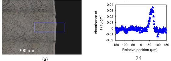
**Figure 1**: a) section of a thick sample exposed during 333 days in contact with a 70 ppm chlorine solution at 40°C, observed by optical microscopy (the blue rectangle corresponds to the analyzed zone by FTIR mapping) b) Carbonyl absorbance through the section in the blue rectangle.
