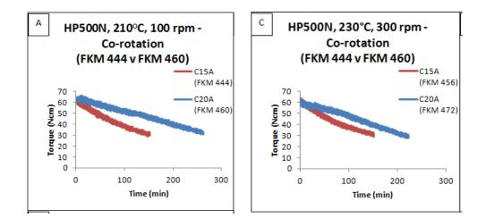
**Fig. 1.** Torque - time history from MR tests for C15A- (lower curves, in red) and C20A- PPNCs produced under different processing conditions.
