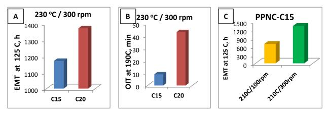
Fig. 2. Time-to-embrittlement from LTTS tests of PPNCs produced under different extrusion conditions.
