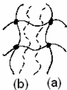
Figure 1. SIPN structure which was obtained by inclusion of linear polyurethane in the cross-linked epoxy resin: (a) polyurethane; (b) epoxy resin based on bisphenol A
