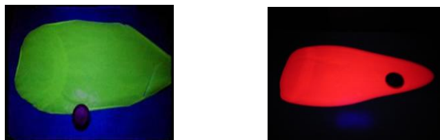
Figure 1.: Photos of polymer /phosphor nanocomposite films under UV excitation
