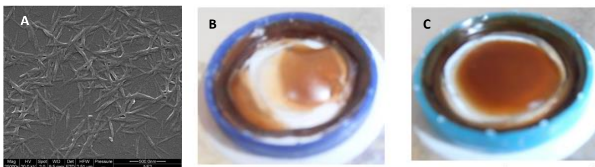
Fig. 1. A. SEM of chitin nanofibrils, B, C. optical view of the air-dried samples of CN and CN/triglycerol (70/30 wt%) thick films
