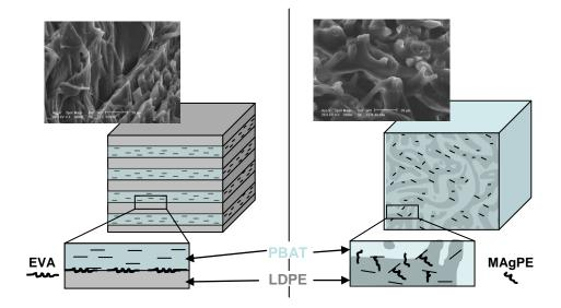
Depending of the compatibilizer, it has been found that the nanoclay can be selectively located in either the polyolefinic or polyester phase while the interphase is invariably stabilized by clay platelets. Remarkably enough, such a selection allows controlling the morphology of the polymer blends. The mechanical properties of the polymer blends were interpreted in the light of their morphology.
